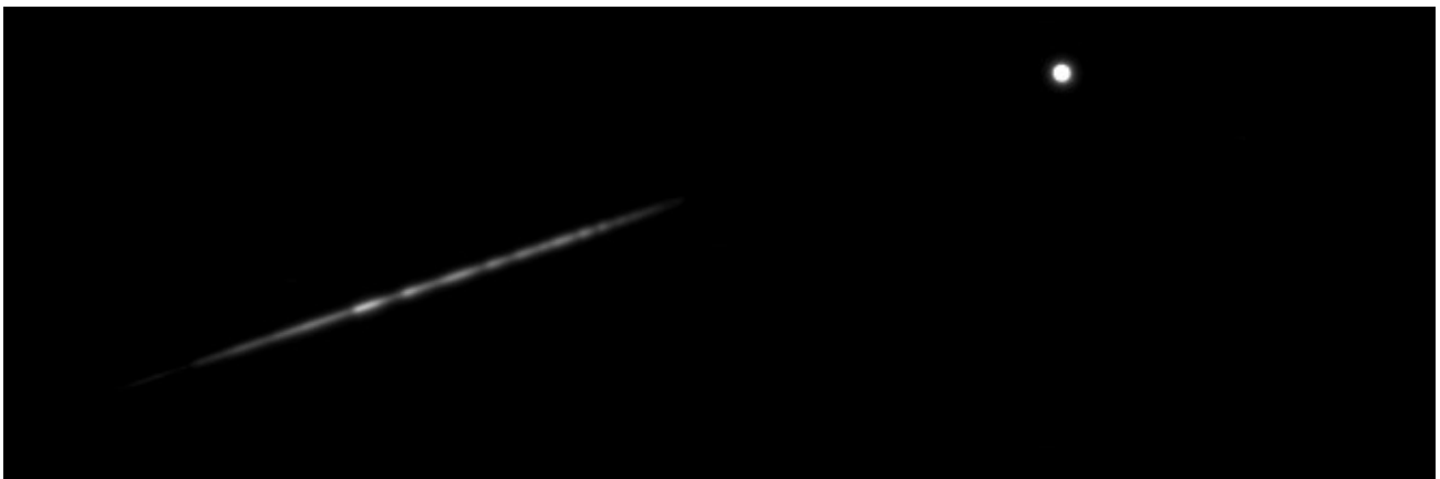
Fig.10: Spectroscopic images already treated (Registax 6.0) from the downloadable files in SASDABA. Top: HD_80493_Alpha_Lyn (K6-III). Bottom: HD_175865_R_Lyr (M5-III). The spectral differences are already visible with a visual examination of the final images. Observations by T. Tobal with the equipment described in this document.
