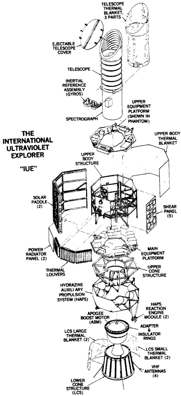
Figure 2-2. IUE Exploded View.
