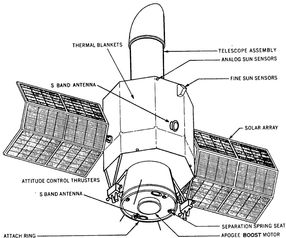
Figure 2-1. IUE Spacecraft in Mission Orbit Configuration.
