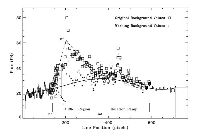
Figure 10.2: Crosscut of background fluxes from a central "Pass 1" swath through an SWP image. Stellar fluxes are off-scale in this diagram. The triangular area describes the local raw background fluxes in the Interorder-Overlap Region where order crowding is severe; the halation region is shown to the right. Small crosses denote the raw fluxes corrected for overlap by the PSF model. The solid line is the Pass 1 solution, a Chebyshev, degree-7 polynomial.
