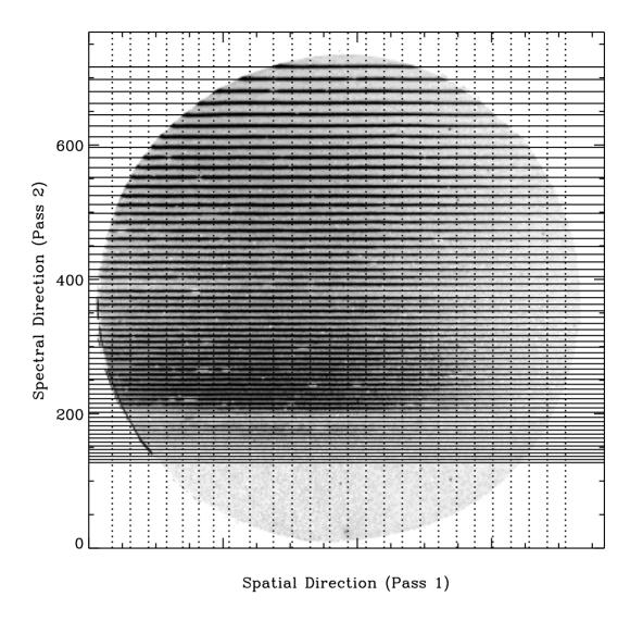
Figure 10.1: Layout of the background extraction swaths on a sample SWP high-dispersion image. Lines running in the vertical (spatial) direction are the Pass 1 extractions. The reconstructed background solutions created in Pass 2 are placed in the positions of the echelle orders (horizontal lines).
